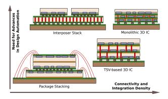
Figure 2: Implementation options for 3D chip stacks. Originating with package stacking, 3D integration has evolved through interposer stacks (also known as "2.5D integration") towards TSV-based and monolithic 3D ICs. Advances in design automation are typically called for the latter two options but are also required for modern, large-scale interposer stacks.
