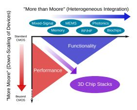
Figure 1: The well-known "More Moore" trend is slowly but surely reaching its limits for CMOS technology. "More than Moore", i.e., exploiting heterogeneous integration, has been identified as novel, important direction. 3D chip stacks offer the potential to meet both trends at the same time.
