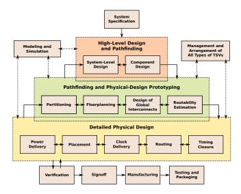
Figure 3: Workflow for designing 3D chip stacks. Pathfinding and prototyping link system-level and IC-level design; this link eases the design closure for the highly iterative process. Modeling and simulation as well as management of TSVs must interact with multiple design stages. Most stages require thermaland variation-aware optimization; feedback loops are essential.
