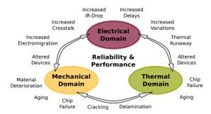
Figure 4: Coupling of various domains in 3D chips, along with potential implications for reliability and performance, require simulation and verification to account for multi-physics effects.
