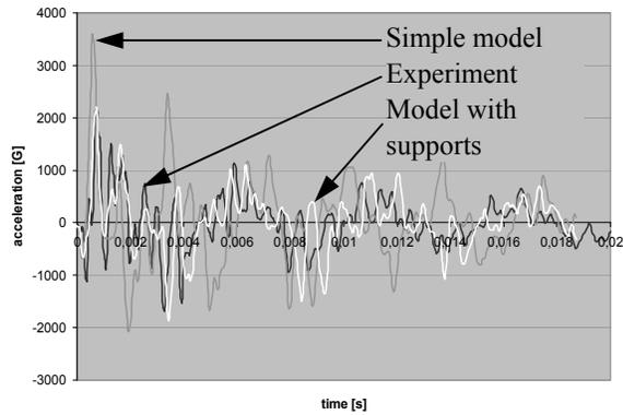
Figure 6: Comparison between experimental PCB vibration behavior and results of different simulation methodologies
