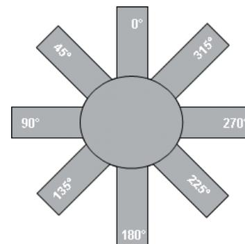
Figure 9: Copper trace orientations at the sub-model copper pads for the investigation of the routing effects
