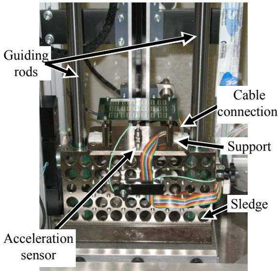
Figure 1: Drop Test setup with guiding rods, base plate, sledge, Jedec PCB, in situ resistance measurement and acceleration sensor
