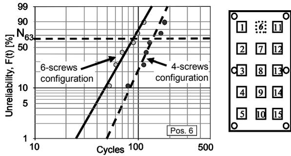
Figure 4: a) Weibull plots of experimental cycles-to-failure of package TFBGA-60 at component position #6 in 4-screws and 6-screws configuration; b) Component positions
