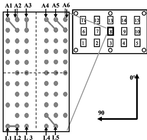
Figure 10: Component orientation and initial pad design at position #8
