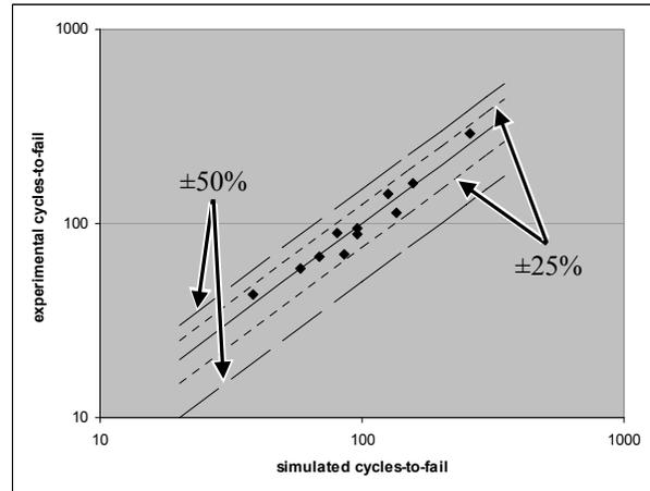
Figure 14: Comparison of simulated and experimental lifetimes
