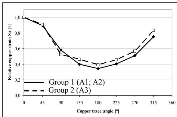
Figure 12: Copper trace routing effect on the relative strain distribution
