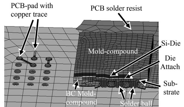
Figure 8: X-section through a TFBGA-60 sub-model with its characteristic features
