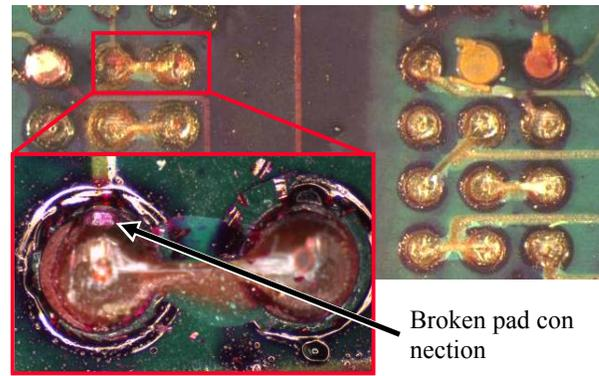
Figure 3: Failure analysis of a JEDEC board with TFBGA-60 packages tested in condition B with 6-screws fixture at component position #8 (see fig. 4b)
