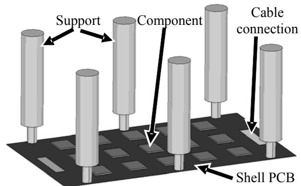
Figure 5: FEM global model of the JEDEC drop test
