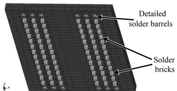
Figure 7: VFBGA-90 component of the global drop test model
