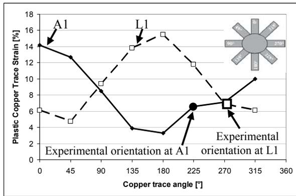
Figure 11: Routing dependent plastic strain of the copper trace at contact interconnection A1 and L1
