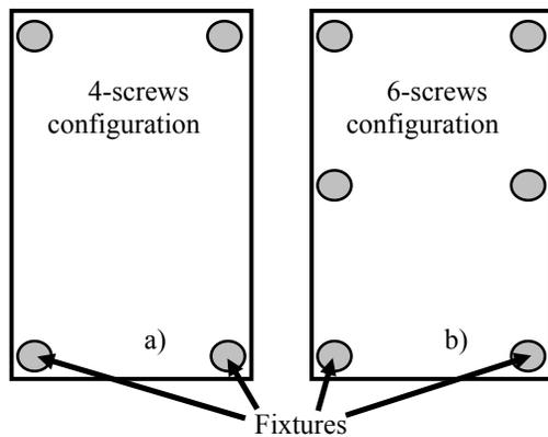
Figure 2: Boundary conditions of the JEDEC board: a) 4-screws configuration according to JEDEC standard; b) 6-screws configuration
